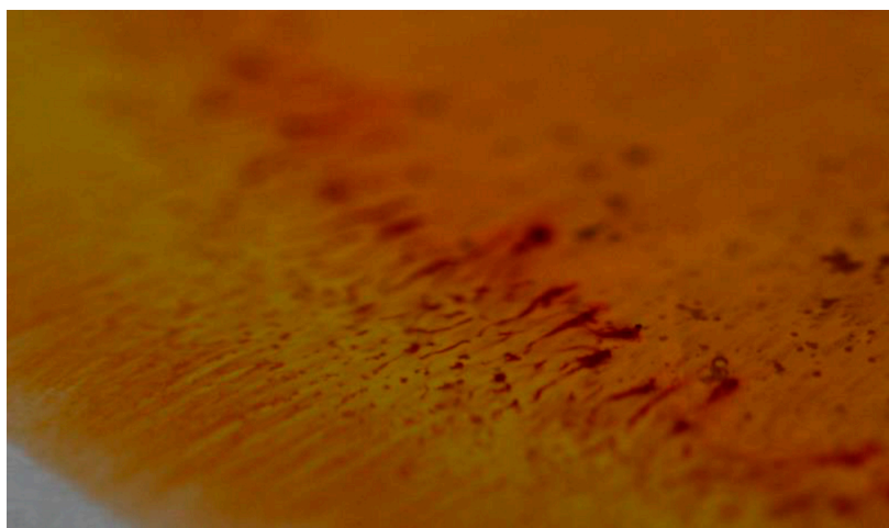
Figure 7. Zoom on the edge of the displacement showing aligned yellow and orange needles in the zone of buoyancy stripes. Behind them, orange red plates develop at the locations where the local mixing due to the convection rolls (see Figure 6b) increases contact between the ROY solution and water.
