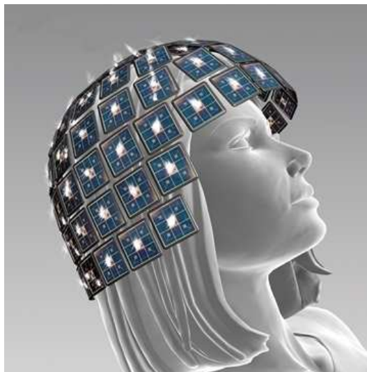
Figure 1.2: Illustration of the measuring of MEG signals via sensors positioned around the head [5].
