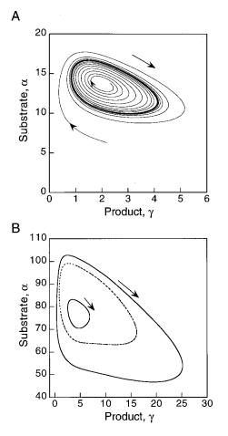
FIG. 2. (A) Limit cycle obtained in the model shown in Fig. 1(A). (B) Birhythmicity in the model of Fig. 1(B); depending on initial conditions, the system evolves toward either one of two stable limit cycles (solid curves) separated by an unstable limit cycle (dashed curve).
