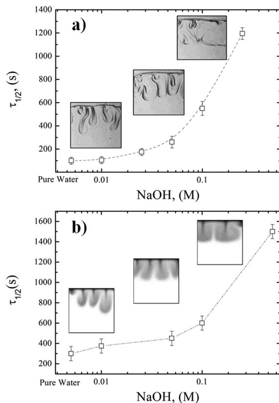
**Figure 4.** Experimental (a) and numerical (b) characteristic time  $\tau_{1/2}$  of the fingers growth as a function of the alkaline concentration of the aqueous phase.
