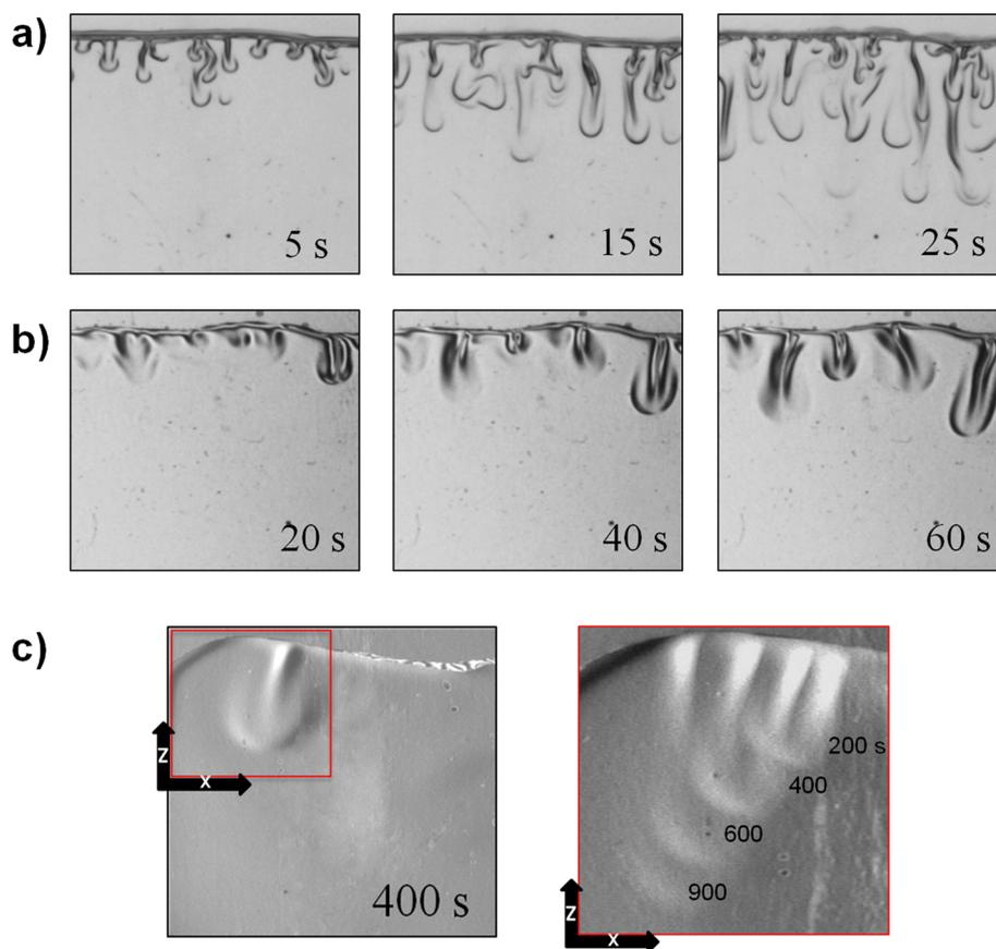
**Figure 1.** Typical density fingering observed experimentally below the horizontal interface between pure water and pure methyl formate (a), ethyl formate, (b) and propyl formate (c). The ester lies on top of the aqueous phase. In (c), the space–time plot in the right panel follows at successive times the vertical growth and the horizontal drifting of the finger shown in the left panel within the red frame of size  $0.95 \text{ cm} \times 0.95$ .
