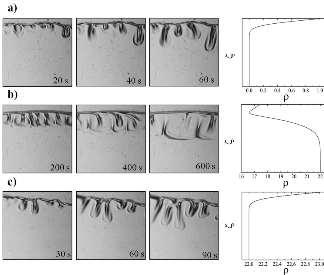
**Figure 3.** Experimental spatiotemporal dynamics below of the interface between ethyl formate and (a) pure water, (b) 1 M NaOH solution, and (c) 1.07 M NaCl solution. In the (b) and (c), the aqueous solutions have the same initial density. The last snapshot of each row shows the asymptotic density profile computed numerically, as described in the text by using  $R_{\text{HCOOEt}} = 1.0$ ,  $R_{\text{NaOH}} \approx 22.0$ ,  $R_{\text{HCOONa}} = 20.5$ , and  $R_{\text{EtOH}} = -4.1$ .
