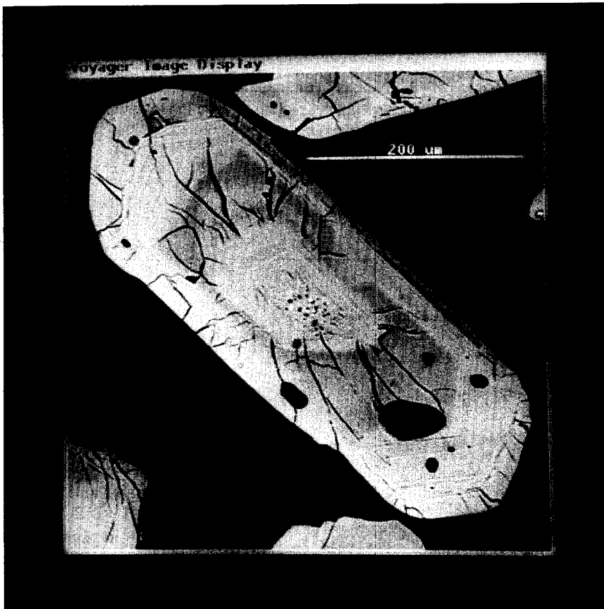
Fig. 2. Photomicrograph (back-scattered image) of zircon grain from sample BB308 used for U–Pb dating. Note the small inner metamict core rich in urano-thorite inclusions, the cracked homogeneous zone, the intensely zoned part (all being of magmatic origin) and the subautomorphic homogeneous rounded external mantle probably of metamorphic origin.
