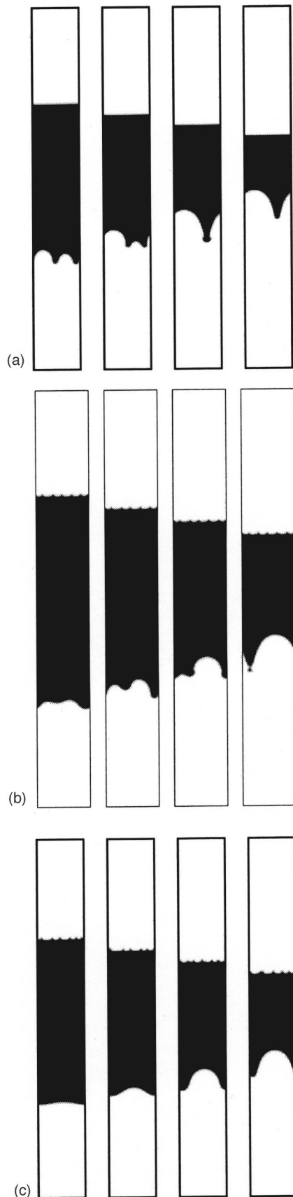
FIG. 8. Nonlinear dynamics of buoyantly unstable exothermic CT fronts with \gamma_T = -2 and four successive times from left to right. In all our numerical experiments the system size is L_y = 512 , L_x = 4096 ; (a) Le = 4 ; (b) Le = 6 ; (c) Le = 8 .
