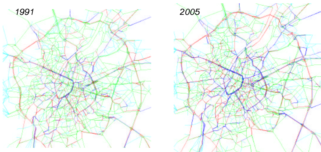
Figure 5.2. Network saturation rate (link intensity vs. link capacity), morning peak-hour
